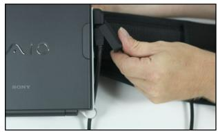
After insertion of the cable close the connector cover.
