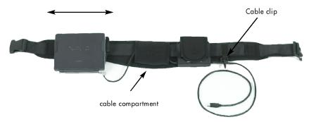
The belt is equipped with a cable compartment between the Vaio and the Power Module where the IEEE 1394 cable can be rolled up thereby adjustet to fit the length of the belt.
