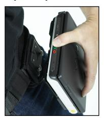
The locking mechanism is quickly released again by pushing the lock button on the top of the belt part of the mounting plate.
