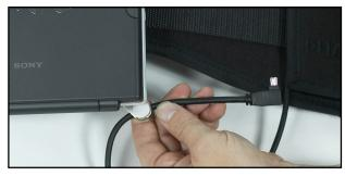
Turn the cable lock 90 degrees and insert the cable in the IEEE 1394 cable connector under the connector cover.
